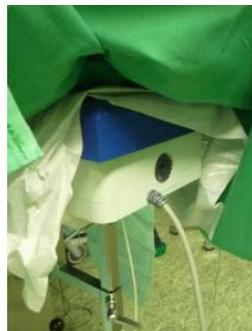
Fig. 2: Navigation head with magnetic field generator
